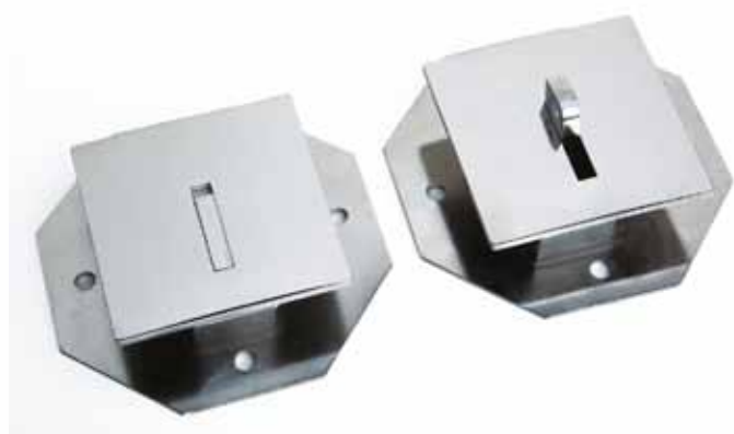
2010002 Multi-functional anchor with hidden eyelet Nicely designed anchor in stainless steel.* Used for in-wall fixations, pool deck anchoring or as an underwater eyelet. This ergonomic anchor has a foldable eyelet, which is hidden when not in use. To be bolted with a face plate 95 x 95 mm and back plate 140 x 140 mm. Anchor depth of 34 mm.
